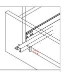
1. Check that the nut is screwed to the bottom.
